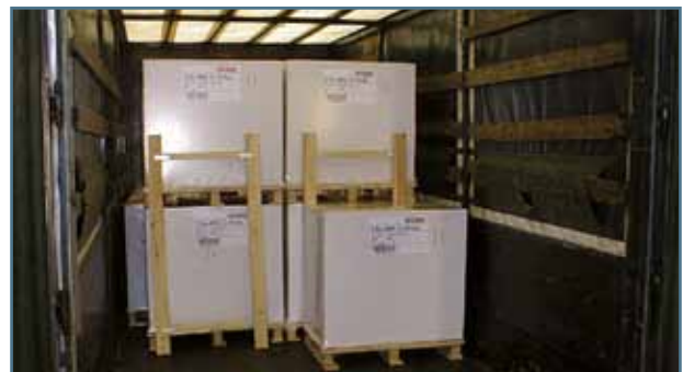
Fig. 18. Panel blocking in forward direction for the second layer
