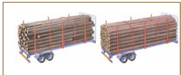
Fig. 66. Load lashing should always add vertical load on round timber
