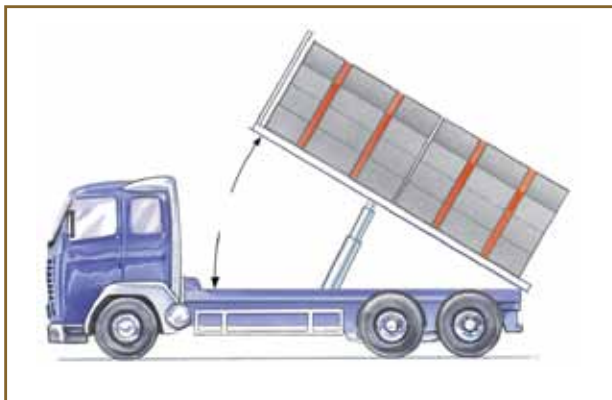
Fig. 11. Practical inclination tests sideways and lengthways
